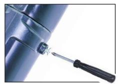
Put a little grease on the screw and tighten it firmly.
