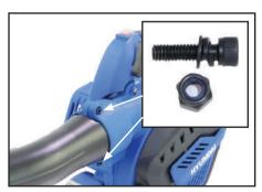
Secure using the M6 Nyloc nuts and bolts. The nuts fit into a hexagonal moulding with the nylon on show.
