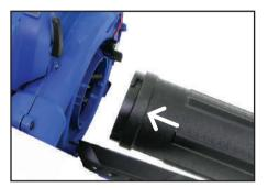
With the moulded keyway at joint with lower pipe at 3 o'clock, engage the collector tube and rotate it anti-clockwise to lock it in place
